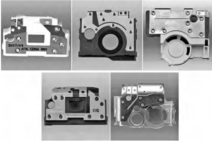
Figure 4.32 Integrated antenna with other components (Reproduced with permission from Shanghai Amphenol Airwave, Inc.)
