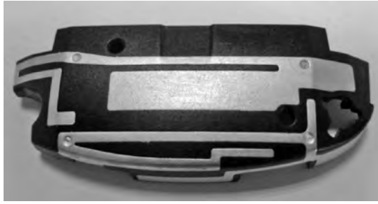
Figure 4.35 Antenna made by DS-MID technology (Reproduced with permission from Shanghai Amphenol Airwave, Inc.)
