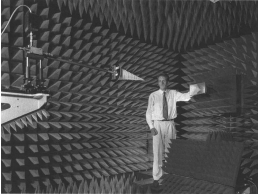
Fig. 15.1 Gain calibration of a log-spiral antenna, being carried out in an anechoic chamber at the National Physical Laboratory, Teddington, UK (Crown copyright).
