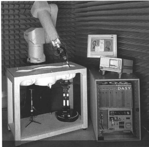
Fig. 15.17 The DASY equipment (photograph: Schmidt and Partner Engineering AG).
